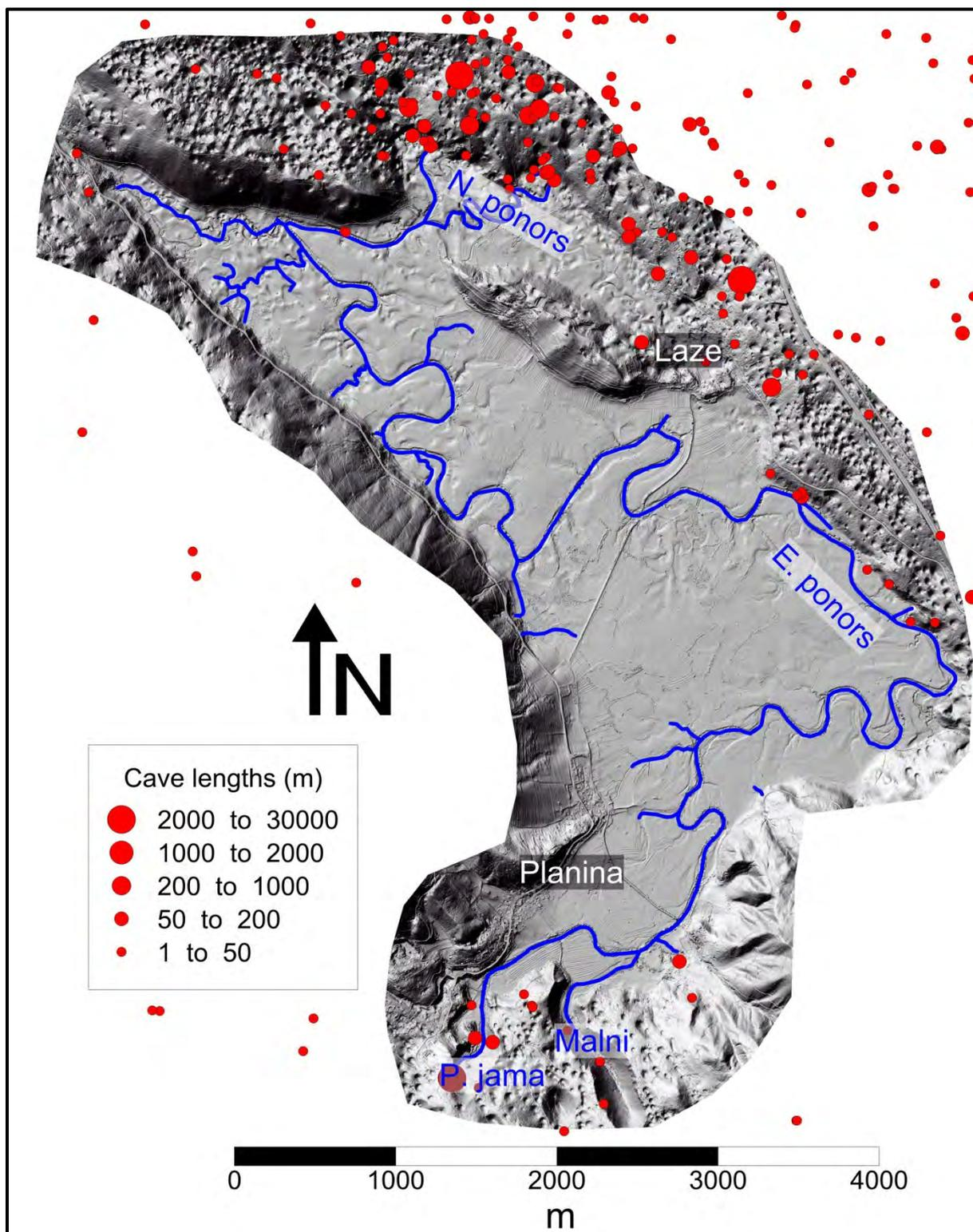
Figure 64: Shaded relief of Planinsko polje with main springs, ponors and flow of Unica river.
