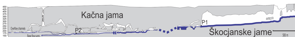
Figure 20: Schematic profile between Škocjanske Jame and Kačna Jama. P1 and P2 indicate the positions of observation points. Blue line shows the flow during low stage. Note the elevated position of overflow channels in Kačna jama.
