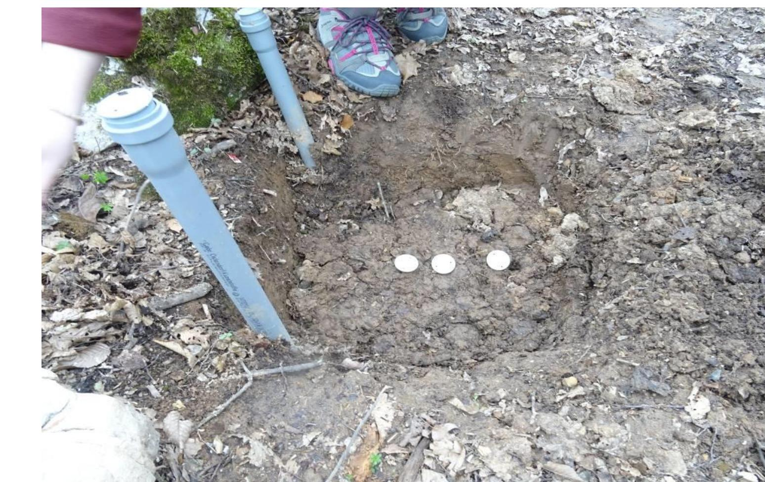
Fig. 3 Placement of Chinese samples on the Jasov plateau at a depth of 20 cm
