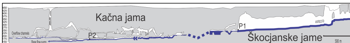
Figure 3.09: Schematic profile between Škocjanske Jame and Kačna Jama. P1 and P2 indicate the positions of observation points. Blueline shows the flow during a low stage. Note the elevated position of overflow channels in Kačna jama.
