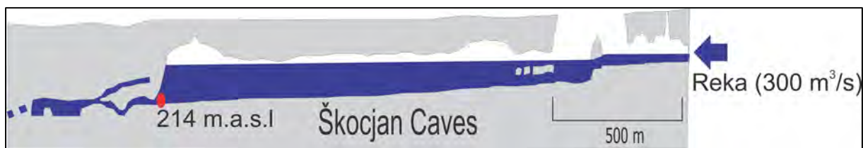
Fig. 3.26: A simplified extended elevation of Škocjan Caves with approximate maximal water level during the flood of February 2019 (from Blatnik et al. 2020).
