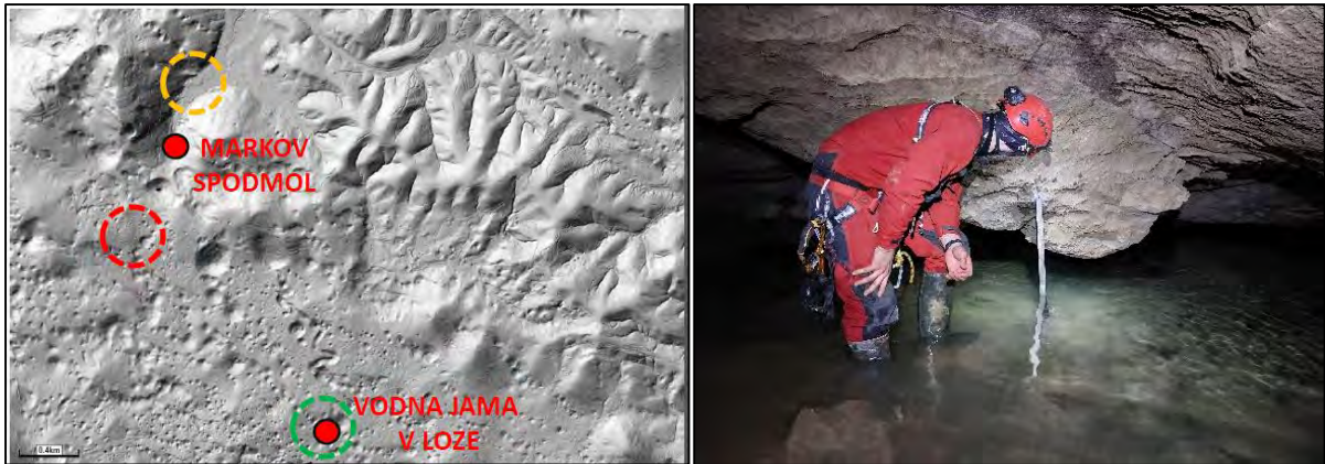
Fig. 1.04: Lidar of the region of Slavinski Ravnik with locations of the three hydrological stations that have been installed – left; hydrological station measuring water level, specific electric conductivity (SEC) and water temperature in the northern part of the cave Vodna Jama v Lozi (Photo: C. Mayaud) – right.
