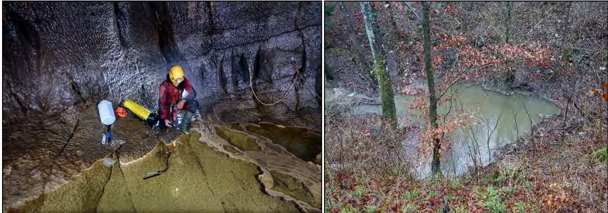
Fig. 1.05: Measuring specific electric conductivity (SEC) and water temperature along the main conduit in the cave Markov Spodmol (Photo: U. Kunaver) – left; flooded swallow hole in front of the cave Markov Spodmol in November 2021 (Photo: C. Mayaud) – right.
