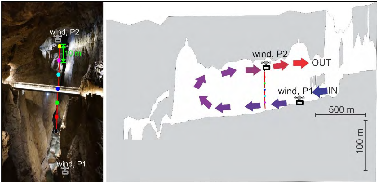
Fig. 3.30: Observations and concept of convection cell in the Reka Canyon in Škocjan Caves (F. Gabrovšek). Left: Picture of Šumeča Jama (Murmoring Cave) and Hanke Channel with position of anemometers (P1-6th Waterfall, P2-Novak Bridge) and line of temperature loggers below P2. Right: Profile of Reka Canyon with (so far) estimated convection cell. Arrows indicate temperature (blue->red = cold -> warm) and direction of airflow.
