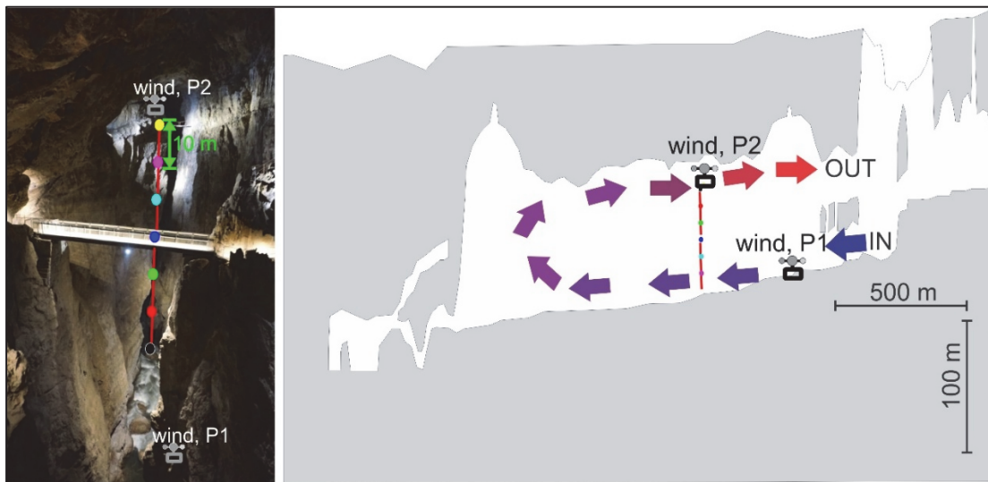
Fig. 1.8: Observations and concept of the convection cell in the Reka Canyon in Škocjan Caves (F. Gabrovšek). Left: Picture of Šumeča Jama (Murmuring Cave) and Hanke Channel with position of anemometers (P1–6 th Waterfall, P2–Novak Bridge) and the line of temperature loggers below P2. Right: Profile of Reka Canyon with (so far) estimated convection cell. Arrows indicate temperature (blue to red = cold to warm) and direction of airflow.
